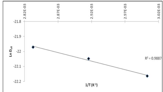
Figure 3. The Arrhenius relationship between the effective diffusivities and temperature
