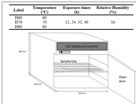
Figure 1. Schematic diagram of humidity chamber with the operating conditions
