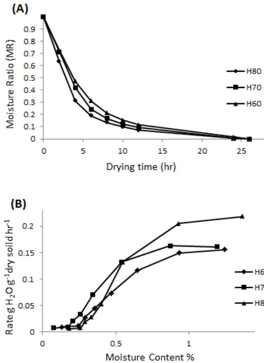
Figure 2. (A) Moisture ratio curves for cocoa beans dried for trials H60, H70 and H80; (B) Drying Rate curves of cocoa for trial H60, H70 and H80 respectively
